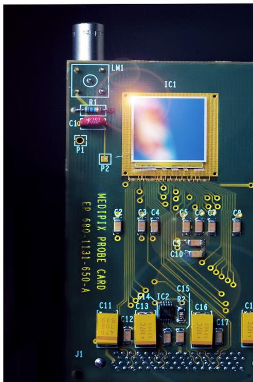
Timepix2 is a programmable, general purpose hybrid pixel detector readout ASIC. The Timepix2 ASIC consists of a matrix of 256x256 pixels with pixel pitch of 55 $\mu$ m, and is applicable to a wide range of applications including X-ray imaging, particle tracking and material analysis.
